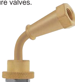
H-6116B High-pressure inflating connection Fits .305-32" thread size with 1/8" NPT female connection with 70° bend. Equipped with hard fiber sealing washer. Used up to 3000 psi working pressure.
