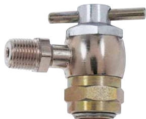
H-556 High-pressure inflating connection Fits .305-32" thread size with 1/8" NPT male connection. Has core depressor pin, and copper sealing washer. Maximum working pressure 3000 psi.
