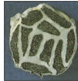
Actual cross-section photo of 5 Tech Permacures which have vulcanized together forming a solid rubber unit.
